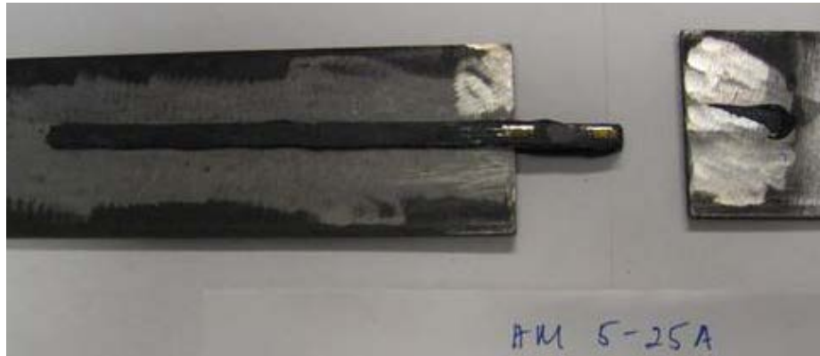
Fig. 2.13: Typical combined steel-epoxy debonding and CFRP delamination seen in ultra high modulus CFRP
