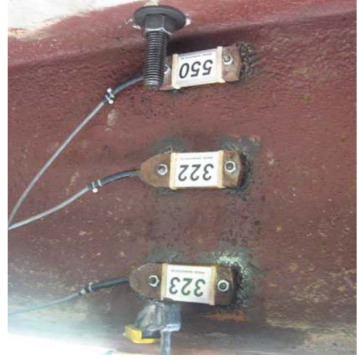
(b) Attached reusable strain gages
