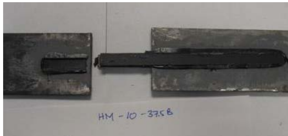
Fig. 2.14: Typical CFRP delamination seen in ultra high modulus CFRP
