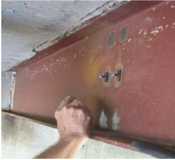
(a) Attaching tabs for gages
