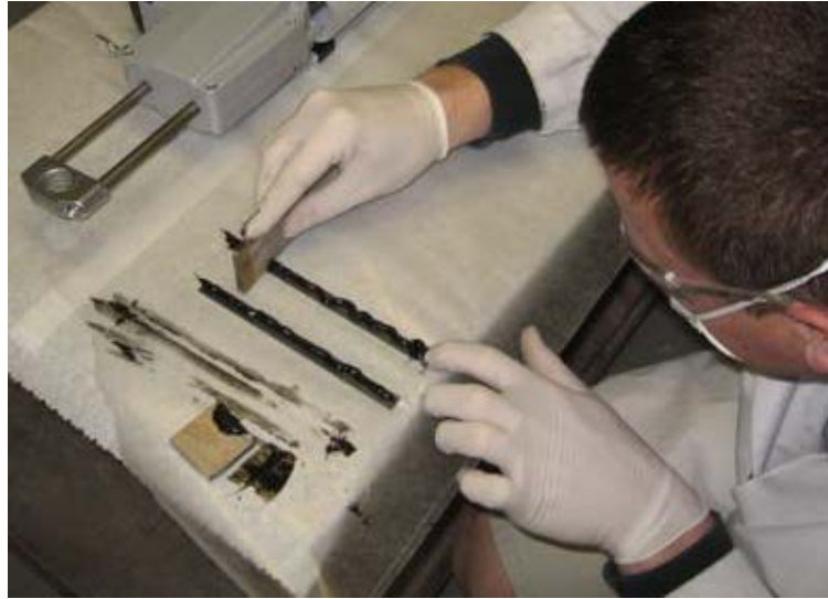
(a) Spreading epoxy on laminate
