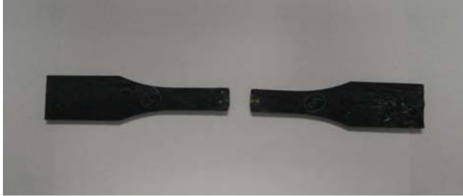
Fig. 2.7: Failure of Epoxy coupons
