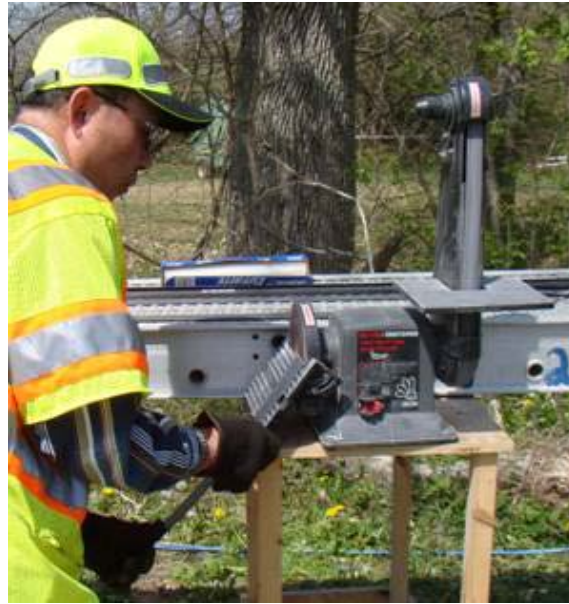
Fig. 5.16: Sanding laminate edges to obtain reverse taper
