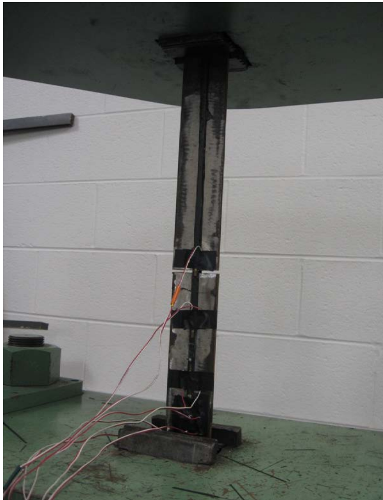
Fig. 2.9: Tensile testing of double strap joint specimen
